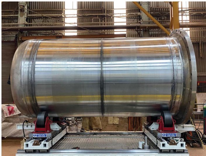
Figure 4: Completed demonstration pressure vessel with two longitudinal and three circumferential weld seams produced using Ebflow. © published courtesy of the EBManPower Project.
