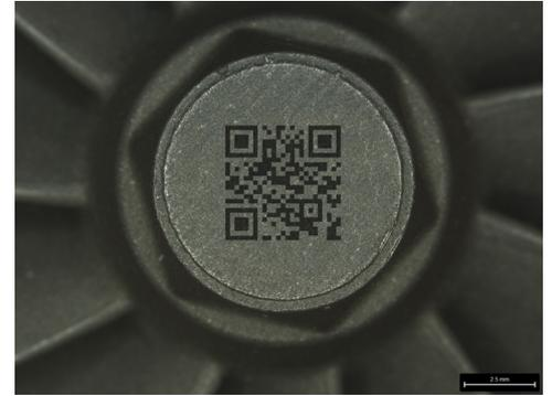
Example automotive components engraved with DMX codes
