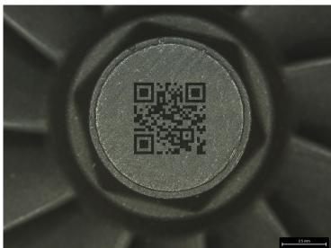
Example automotive components engraved with DMX codes
