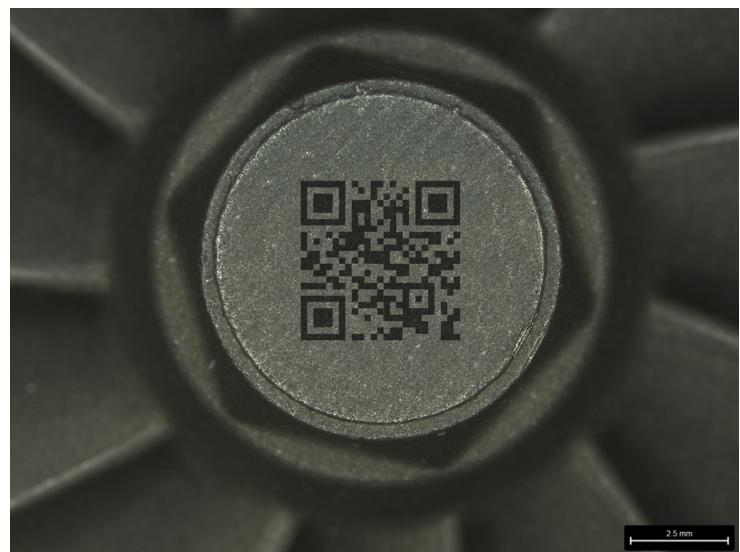
Example automotive components engraved with DMX codes
