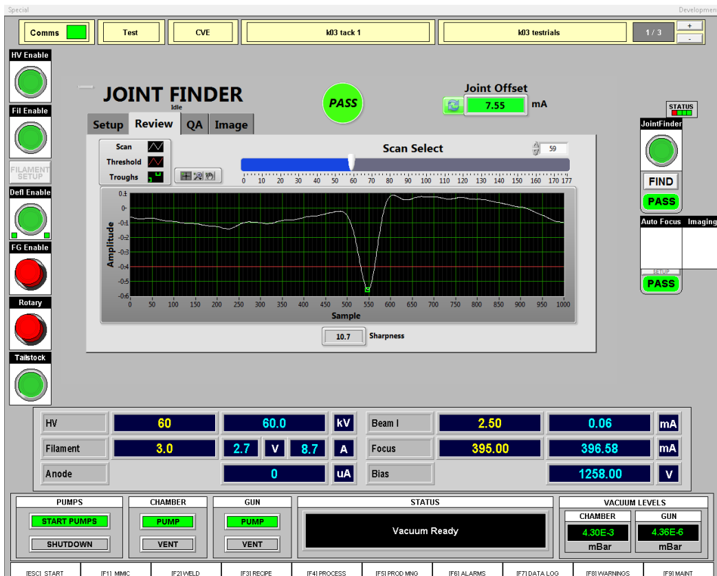
Joint finding control system
