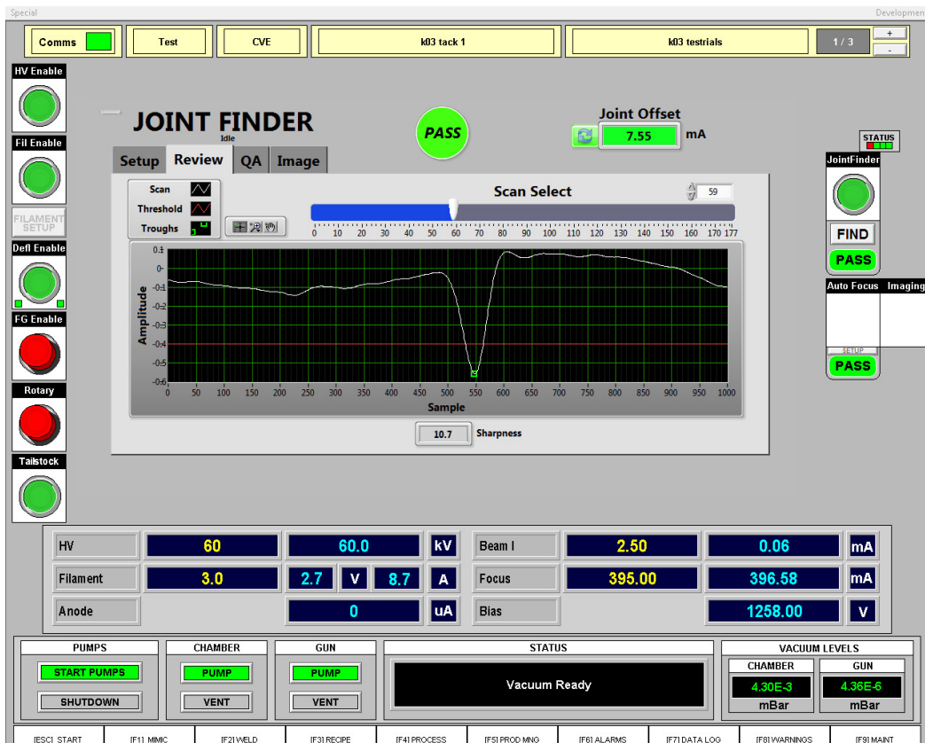
Joint finding control system
