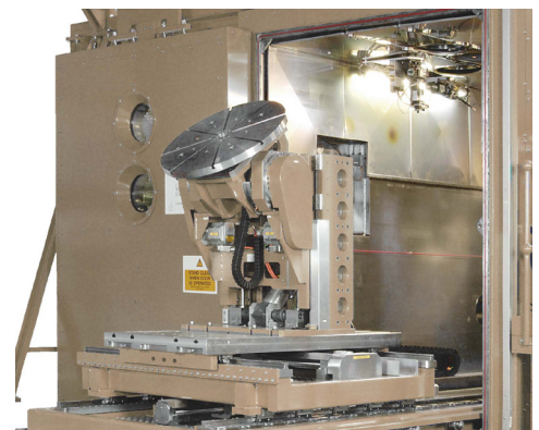
Rotary tilt headstock and tail- stock fixed on an XY table
