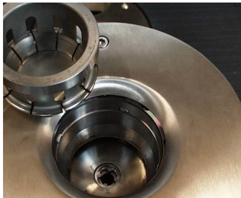
Dual drive tooling housing, shaft adapter and wheel collet
